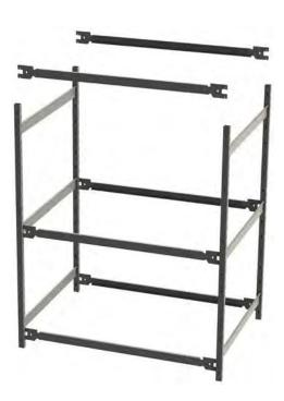
To install the beams, insert one end of the beam past the notices in order to leave enough space for the other end to clear the post and slide into place. Align the notches once both sides are in the slots of the post. Use a rubber mallet to secure the beam in place.
