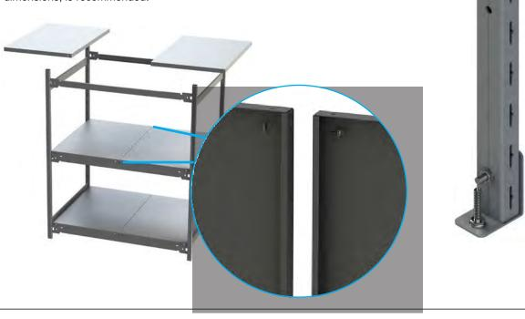
To join 2 posts vertically, bolt a splice bracket to either side of the posts at the joint. When splicing back-to-back units, only 1 more splice bracket is required.
